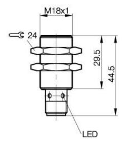
Inductive Sensors BES 516-355-E5-Y-S 4 M18x1 x 44.5 normally-open Sn=5mm shielded
